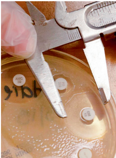
The use of calipers to measure the zone of inhibition.
