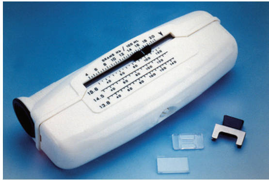
Fig. 9.9 The hemoglobinometer uses a color-matching method to determine the hemoglobin concentration in a sample of lysed red blood cells.
