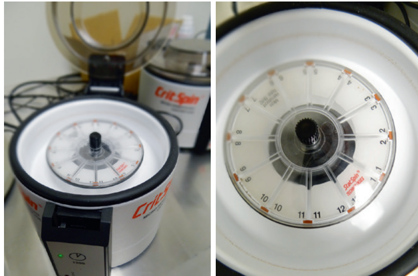
A microhematocrit centrifuge designed for small-capacity tubes.
