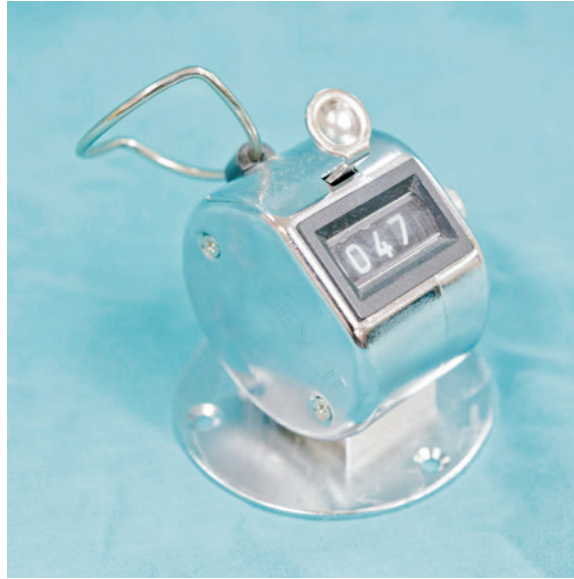
The hand tally counter is used to keep track of numbers of cells counted.
