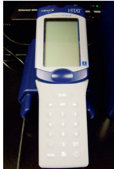
The i-STAT analyzer has cartridges that are used for the performance of coagulation tests.
