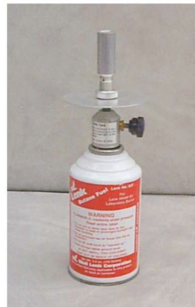
Fig. 38.3 Propane burner for sterilizing metal inoculating loops. (Courtesy
