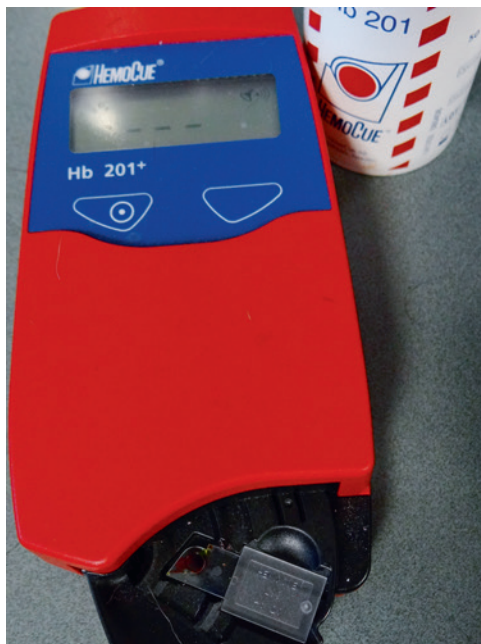
Fig. 9.10 The HemoCue is a type of photometer that is used to measure
