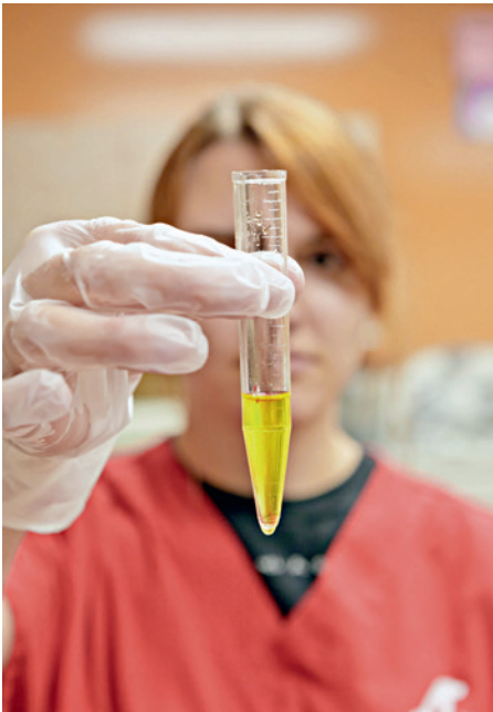
Conical Centrifuge Tube. This type of tube is used to centrifuge substances that contain solid material in solution.
