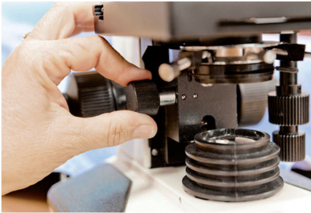
The substage condenser control is used to raise and lower the
