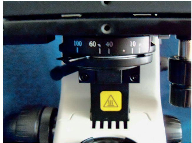
Fig. 3.6 The aperture diaphragm controls the amount of light illuminat
